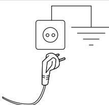
The power supply cable must be easily accessible after installing the appliance.
